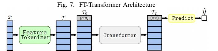
As stated in the original paper, FT-Transformer uses pre-normalization, which differs from post-normalization in that the input will be added with the output of multi-head self-attention (MHSA) directly without normalization. Another detail worth noting is that the first Transformer layer will skip the first normalization given that the experiment results conducted by the original authors showed that this could improve the performance of FT-Transformer significantly.
